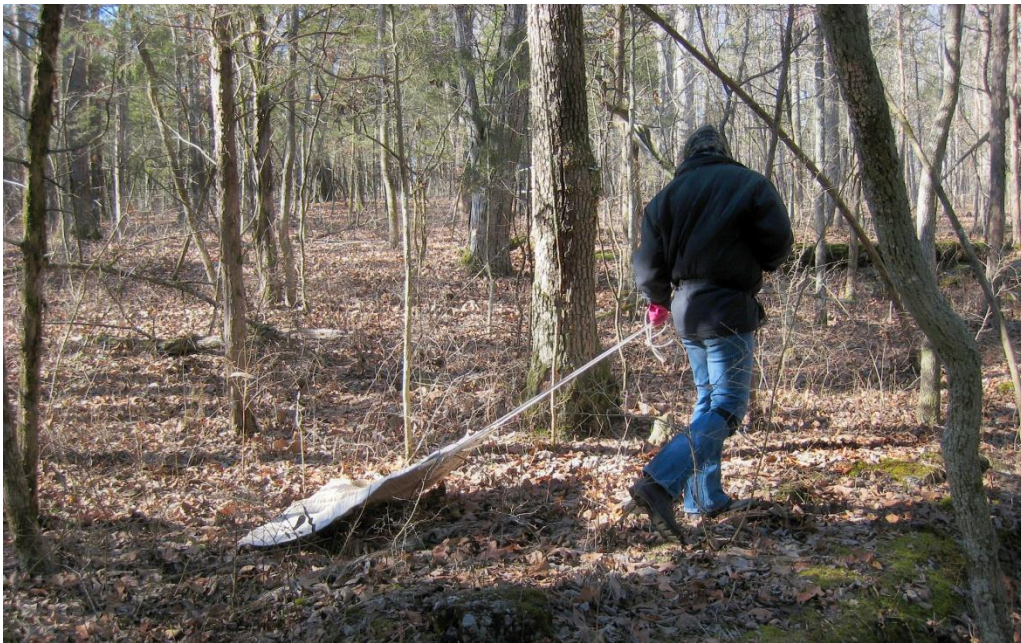
Figure 3.2: Drag sampling at Henry Horton State Park, Tennessee, in January 2008.
